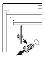
4. Feed sensor through opening and secure sensor cable with strain relief device.
